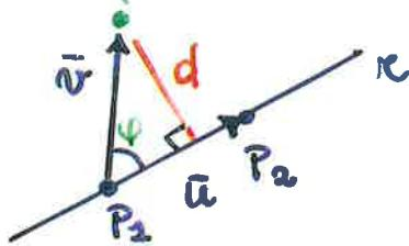
$$d = v \sin \varphi = \frac{v u \sin \varphi}{u} = \boxed{\frac{|\bar{u} \times \bar{v}|}{|\bar{u}|}}$$
