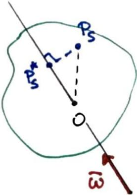
$$\bar{\omega} \times (\vec{r}_S - \vec{O}) = \bar{\omega} \times (\vec{r}_S - \vec{r}_S^*) + \bar{\omega} \times (\vec{r}_S^* - \vec{O})$$
